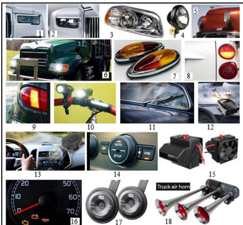
1-6- car head light and spotlight 7-9- Car's turn signal, tail lamps 10- bicycle headlight 11- windscreen-wiper 12-15 car defroster ,demister, fan heater 16- Dashboard oil pressure warning light 17-car horn 18- truck air horn .
