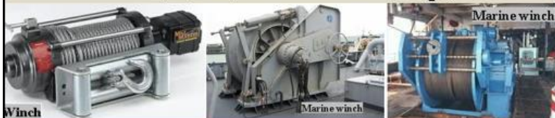
Marine winches and capstans for operating cargo lifting gear, raising anchor
